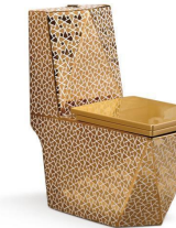
A8030G3 WASHDOWN/SIPHONIC ONE-PIECE TOILET Size:690×370×840mm S-trap:250/300mm Roughing-in P-trap:180mm Roughing-in
