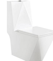
A8030 Washdown one-piece toilet Size : 690×375×830mm S-trap:250mm Roughing-in P-trap:180mm Roughing-in
