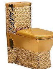
A8050G3 Washdown one piece toilet Size: 720 × 390 × 780mm S-trap: 250mm Roughing-in P-trap: 180mm Roughing-in
