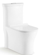
A8045 WASHDOWN/4D EDDY ONE-PIECE TOILET Size:660×370×735mm S-trap:250/300/400mm Roughing-in P-trap:180mm Roughing-in
