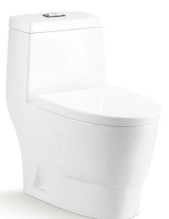
A8048 WASHDOWN/EDDY ONE-PIECE TOILET Size:700×400×710mm S-trap:250/300/400mm Roughing-in P-trap:180mm Roughing-in
