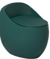
A8115G Washdown one piece toilet Size: 690 × 470 × 610mm S-trap: 300/400mm Roughing-in P-trap: 180mm Roughing-in
