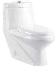
A8011 WASHDOWN ONE-PIECE TOILET Size:700×430×730mm S-trap:250mm Roughing-in P-trap:180mm Roughing-in
