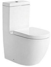
A8120 Washdown one piece toilet Size: 670 × 370 × 840mm S-trap: 250mm Roughing-in P-trap: 180mm Roughing-in
