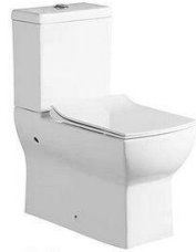
B8111 Washdown two piece toilet Size: 640 × 370 × 800mm S-trap: 100/250mm Roughing-in P-trap: 180mm Roughing-in
