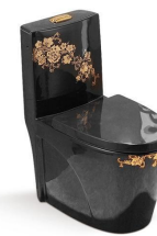
A8020BG WASHDOWN/SIPHONIC ONE-PIECE TOILET Size:680×385×780mm S-trap:250/300mm Roughing-in P-trap:180mm Roughing-in
