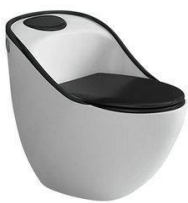
898-2 Washdown one piece toilet Size: 690 × 660 × 420mm S-trap: 250mm Roughing-in P-trap: 180mm Roughing-in
