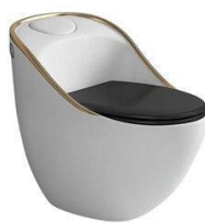
898-1 Washdown one piece toilet Size: 690 × 660 × 420mm S-trap: 250mm Roughing-in P-trap: 180mm Roughing-in
